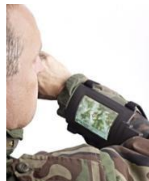
A wrist mounted flexible OLED display and communications device built on thin metal foil, which uses Universal Display's highly efficient phosphorescent OLED technology and materials.
